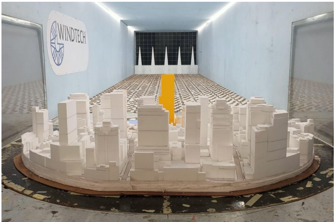
Figure 2e: Photograph of the Wind Tunnel Model Envelope Case, view from the east
