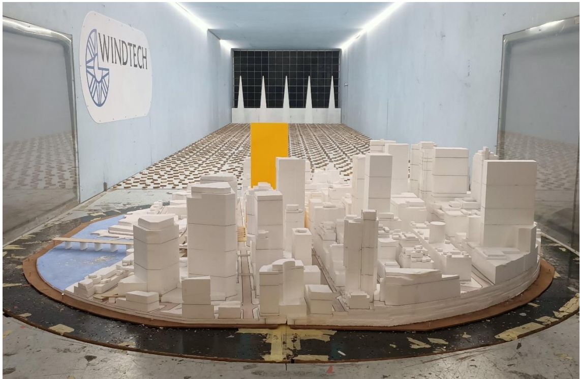
Figure 2d: Photograph of the Wind Tunnel Model Envelope Case, view from the south
